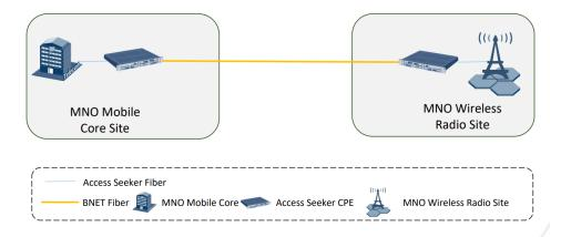
The CPE (Access Seeker CPE) can be provided either by the Access Provider or by the Access Seeker (at the Access Seeker's choice)
