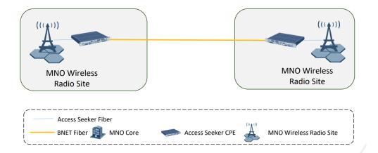
The CPE (Access Seeker CPE) can be provided either by the Access Provider or by the Access Seeker (at the Access Seeker's choice)
